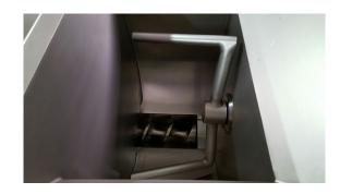
Hopper capacity approx. 300 litres (mixing capacity approx. 150 kg)
