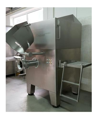
Mixing Grinder 160 mm hole plate diameter Almost completely made of solid stainless steel 2-speed working worm
