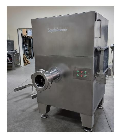
Mixing Grinder 200 mm hole plate diameter Almost completely made of solid stainless steel 2-speed working worm3-phase motor IP 55, completely closed, approx.25/37 kW1-speed mixing paddle motor, approx. 1,5 kW with
