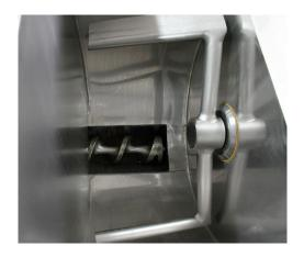
Hopper capacity approx. 300 litres (mixing capacity approx. 150 kg) Worm, worm housing and closing nut completely stainless Elongated feet for higher outlet for loading trolleys BW 200 Integrated lifting device, for standard meat bins
