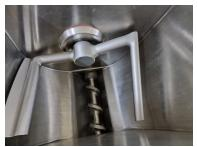
3-phase motor IP 55, completely closed, approx. 14/18 kW 1-speed mixing paddle motor, approx. 1,5 kW with 2 mixing arms, independent of working worm, Hopper capacity approx. 170 litres (mixing capacity approx. 100 kg)
