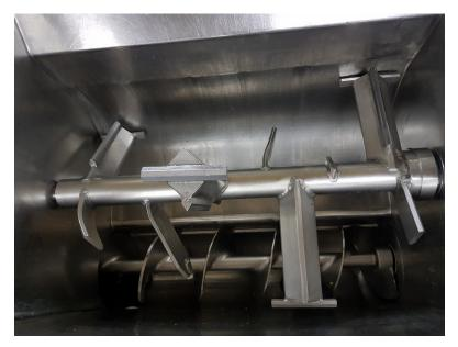
Working worm Machine dimensions in cm: Width: 215,0 Depth: 150,0 Height: 196,0 Main Motor Power: 45 kW Installed Power approx. 65 kW Voltage: 380 V, 50 Hz
