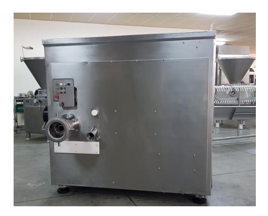
Type: KRAMER + GREBE MW 200 Completely made of special stainless steel Specialized for grinding cheese and yellow cheese BLOCKS Hole plate diameter: 200 mm Hopper capacity: approx. 400 liters
