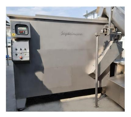
Hopper volume : 2 500 liters Mixing capacity: approx. 1400 kg 2 separate reduction gears with electrical motors two mixing shafts with paddles, parallel 2 exhaust openings of the funnel
