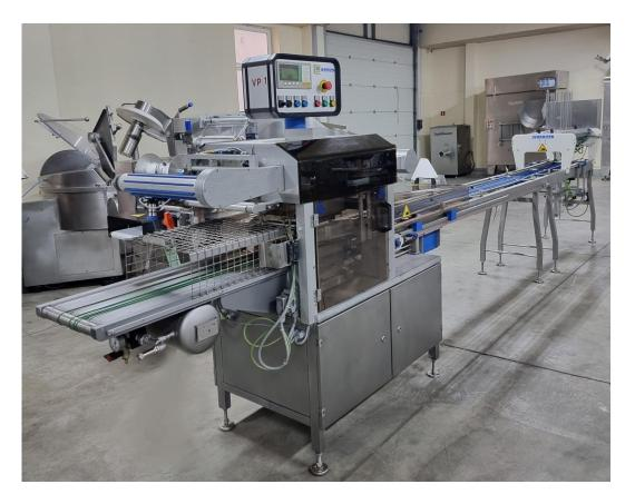
Traysealer SEALPAC 350 is made of speacial stainless steel and operates with servo motors. It's appropriate for packing of large amount of products, with or without gas.
