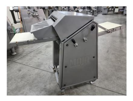
The automatic MAJA derinding machines ESB 4434 are made for the safe derinding of flat meat cuts through an infeed conveyor belt.
