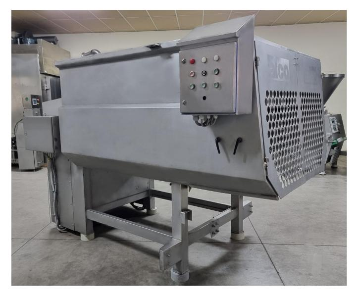
Hopper volume : 2200 liters Mixing capacity: approx. 1100 kg 2 separate reduction gears with electrical motors two mixing shafts with ribbons, parallel
