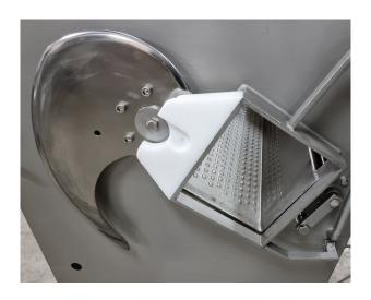
Cutting length adjustable hydraulic Automatic return of the bracket
