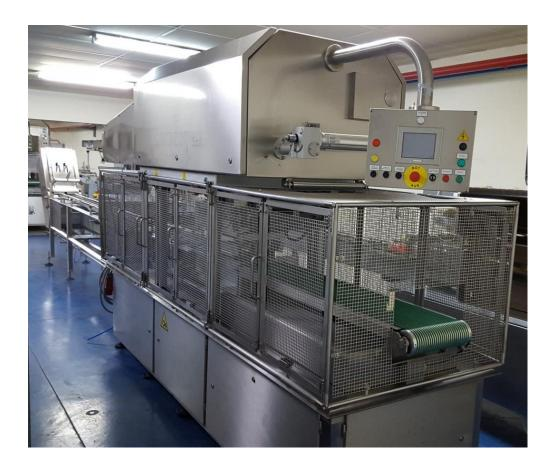
The traysealer MONDINI is completely made of special stainless steel. It's appropriate for packing of large amount of products, with or without gas **Standard accessories MONDINI E 365 VG**
