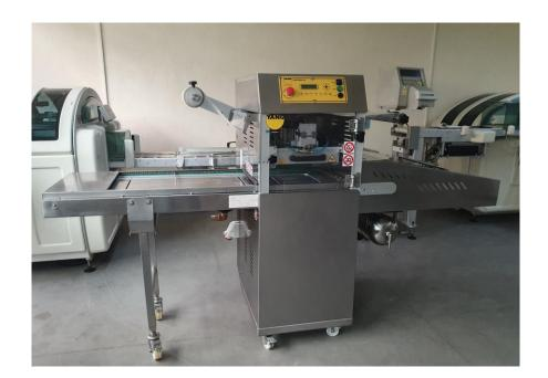
Traysealer YANG is made of speacial stainless steel and operates with servo motors. It's appropriate for packing of large amount of products, with or without gas.
