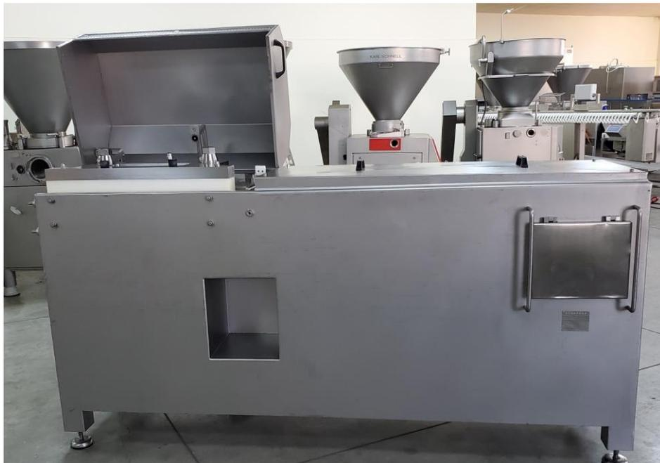
The main area of use of the HAMAX 800 whole muscle stuffer is automatic filling of fresh (for example, as restructured meat) or cured meat parts/pieces of meat (for example, as raw and cooked curedmeat) in plastic casings and nettings. The fundamental principle of the machine is based on a hydraulically driven piston that presses the meat into the casings.
