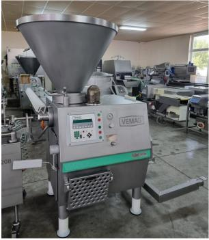
Continuous vacuum filler for straight filling and portioning
