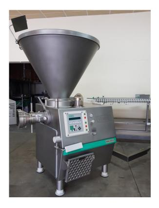
Continuous vacuum filler for straight filling and portioning
