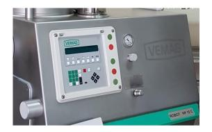
program memory for 99 filling programs, Portion weight: from 5 up to 60 000 g VEMAG DuoDrive with separate drive for double screw and feed: double screw drive
