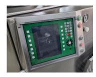
program memory for 99 filling programs, portioning weights can be set from 1 to 99,999 grammes, portioning speed > 700 portions/minute, depending on weight,
