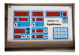
For set and actual value of the revolution of the knife shaft, speeds, working time, temperature, vacuum, with buttons for adjustment
