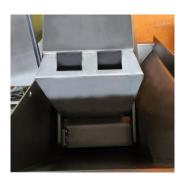
Hydraulic worm ejector, manually operated
