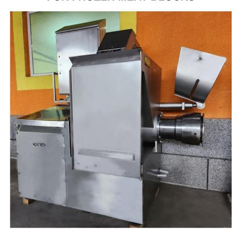
300 mm hole plate diameter Almost completely made of solid stainless steel For frozen meat blocks till maximum 900 x 500 x 150 mm
