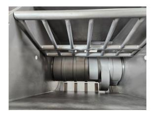
Rotating crushing rollers for several seconds cope with blocks of meat frozen to -30 ° C. For optimum processing quality, block temperatures between -12 ° C and -20 ° C are recommended.
