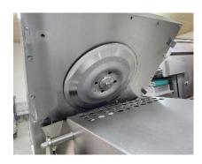
Transport conveyor for transporting sliced portions. The transport conveyor is attached to the Slicer on the infeed side and is supported by the floor or by a packaging machine on the discharge side. The conveyor belt can be easily removed from the belt frame for cleaning. The transport speed is controlled by the Slicer.
