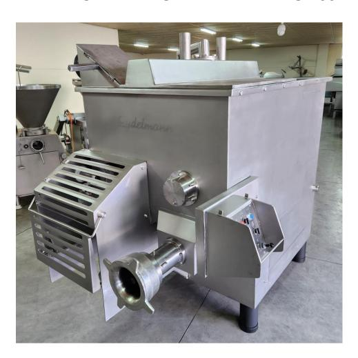
200 mm hole plate diameter Almost completely made of solid stainless steel 2-speed working worm, motor approx. 25/37 kW
