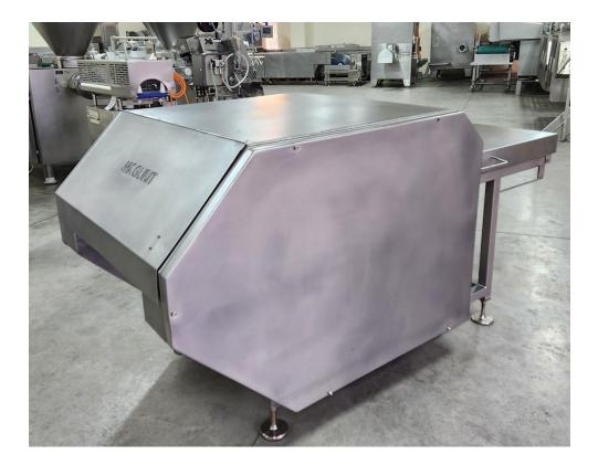
Type: Magurit - 345 - rotary Max. width of cutting: 520 mm Max. height of cutting: 250 mm Max. length of the meat block: 600 mm Temperature of the meat block: up to– 25° C Control panel mounted on the machine
