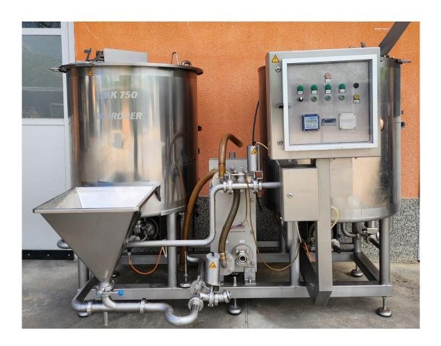
The LMK 750-2 mixer is used for the precise mixing of solid and liquid components. The operations are automatically controlled up to the completely mixed brine.
