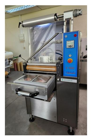
Semi-automatic traysealer Including Vacuum/gas system Build-in vacuum pump Productivity: 3-5 tatcs
