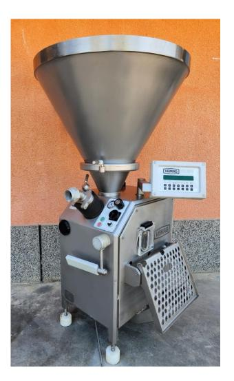
**VEMAG ROBOT 500** type 128/230 - Continuous vacuum filler for straight filling and portioning
