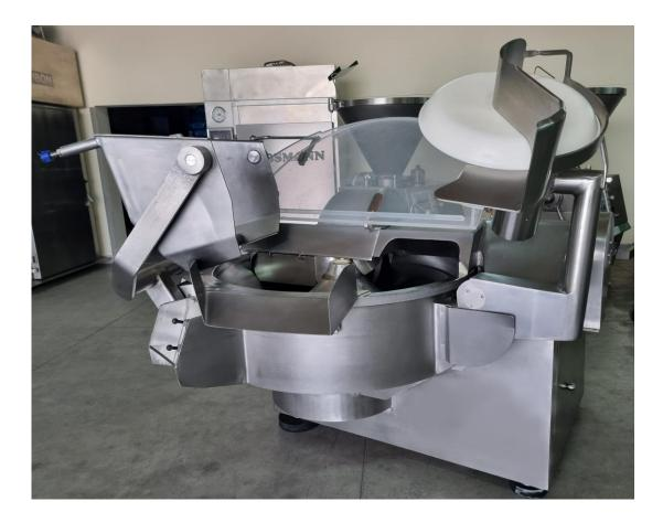
6 steplessly adjustable knife speeds2 separate bowl speeds2 mixing speedsCompletely made of special stainless steel
