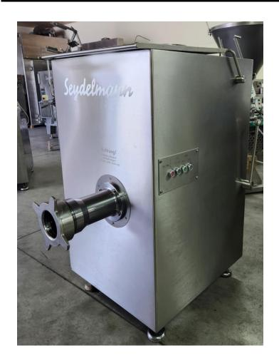
130 mm hole plate diameter Almost completely made of solid stainless steel 2-speed working worm
