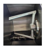
Hopper capacity approx. 170 litres (mixing capacity approx. 100 kg)
