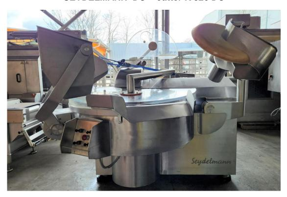
6 steplessly adjustable knife speeds 2 separate bowl speeds
