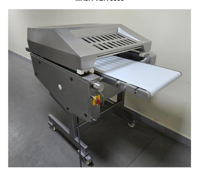
The automatic MAJA derinding machines are made for the safe derinding of flat meat cuts through an infeed conveyor belt.
