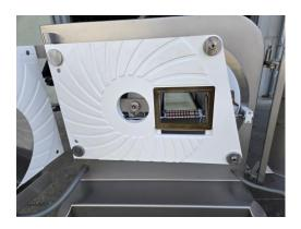
The FALCON uses a 360° scanner instead of conventional mould technology
